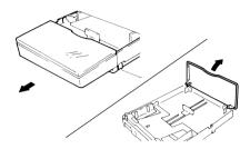
Press down the Paper Lifting Plate until it locks. Fan the paper stack thoroughly, align the edges, and place the paper in the cassette.
